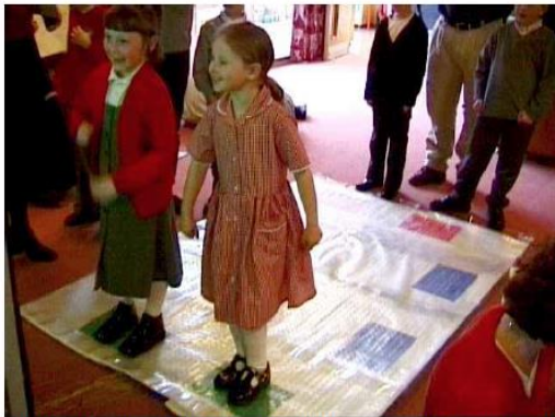
Figure 2: second prototype magic carpet with rectangles to show positions of sensor pads (see color plate on page 00)
